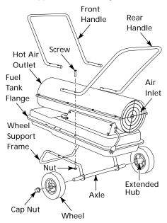
Figure 4 - Wheel and Handle Assembly
